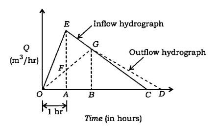
Determine the channel storage after one hour (i.e., under the peak of inflow hydrograph) and the maximum storage and the time at which it occurs along with the principle on which these are computed.
