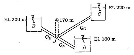
The water surface elevations in the reservoirs and the piezometric head at junction J are indicated in the figure. Write the mass balance equation at junction J and justify the answer.
